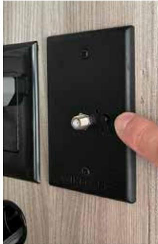
Antenna/Cable push-button selection switch with green LED
