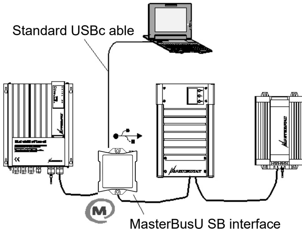
Typical MasterBus communications network showing a PC connected via a MasterBus USB Interface module.
