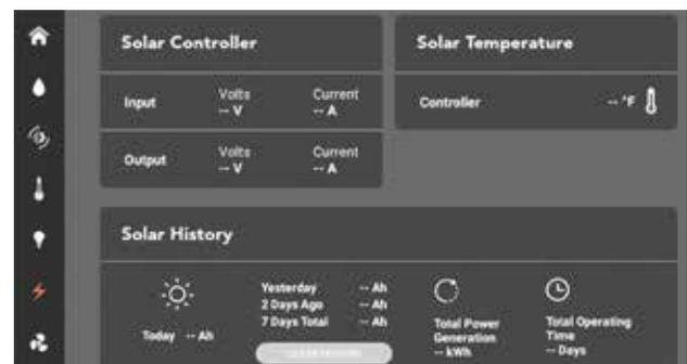
**NOTE:** The Solar Charging System Controller is powered directly from the auxiliary battery(ies), therefore, it is ON regardless of the position of the Master Battery Switch.
