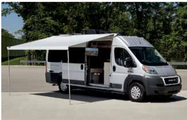
The patio awning operates from the motorhome's 12-volt DC electrical supply. The master battery switch will need to be ON prior to operating the awning.
