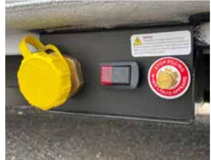
The main propane gas valve installed on this vehicle is controlled by an electrical solenoid. The actuation switch for the gas valve is located on the propane access panel, positioned along the lower left side of the vehicle. This panel also contains the propane tank fill port and a propane tank bleeder valve.
