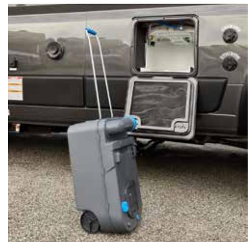
**NOTE:** Some Class B motorhomes have a bathroom with a cartridge toilet located at the rear of the vehicle. Access to the toilet cartridge is through the rear door.
