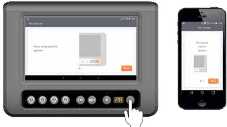
3. Using the < or > buttons on the Master Controller, navigate to the 'PA' menu item.
