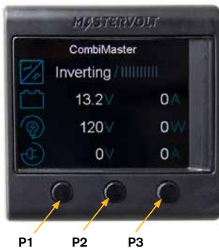
Mastervolt SmartRemote Inverter Monitor and Remote Controller
