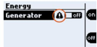
NOTE: A generator warning will appear if the generator fault LED is actively blinking.
