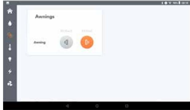
As a safety precaution, the RVMaster App will disable all motor control if the vehicle's ignition is ON. This safety feature prevents any accidental operation of the motors while you are driving the vehicle.
