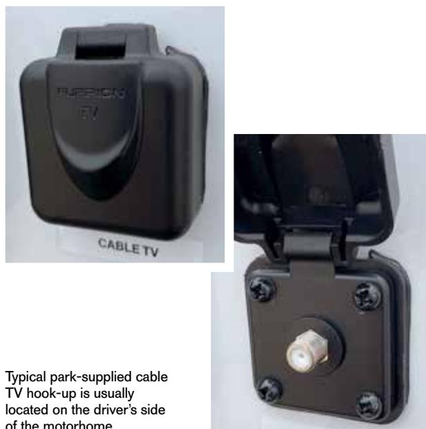
Typical park-supplied cable TV hook-up is usually located on the driver's side of the motorhome.
