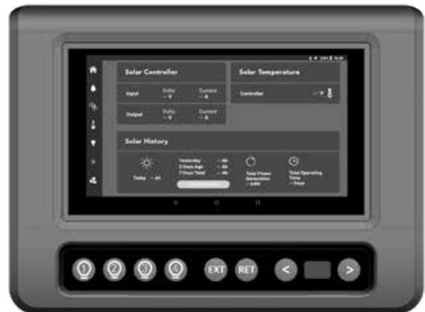
Illustration of BMPPro touchscreen panel showing remote solar charging screen. Through the touchscreen panel, solar charging and battery charge condition can be monitored. Solar controller set-up is accessed through the Settings Menu.
