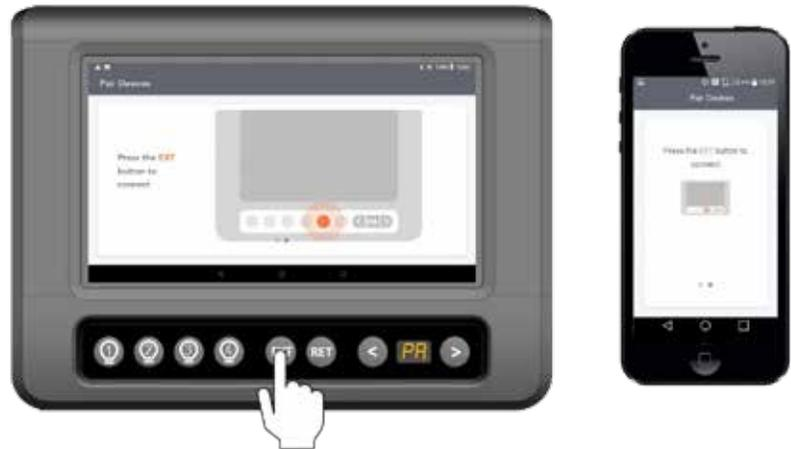
5. When pairing is successful, the PA indicator will turn OFF, indicating the process is complete. The touchscreen on your smartphone or tablet should now have the same display as the Rapid Camp+ Touchscreen Panel.
