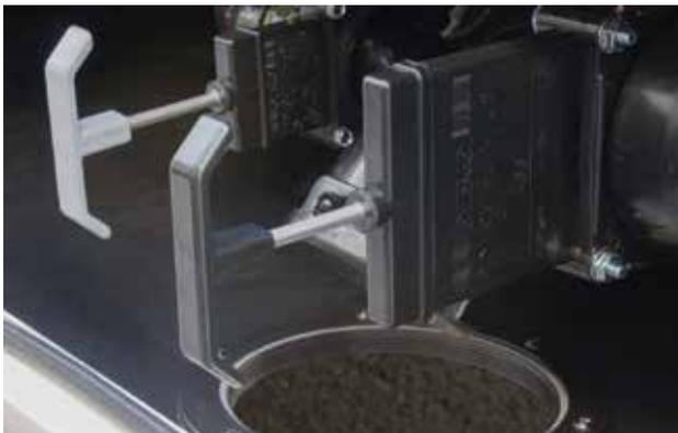
Typical termination valve configuration
