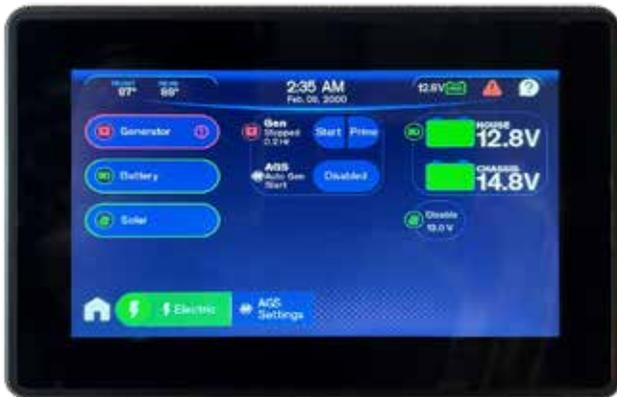
Typical multiplex main control panel. Electrical system monitoring is usually located on the main menu (Home) screen.
