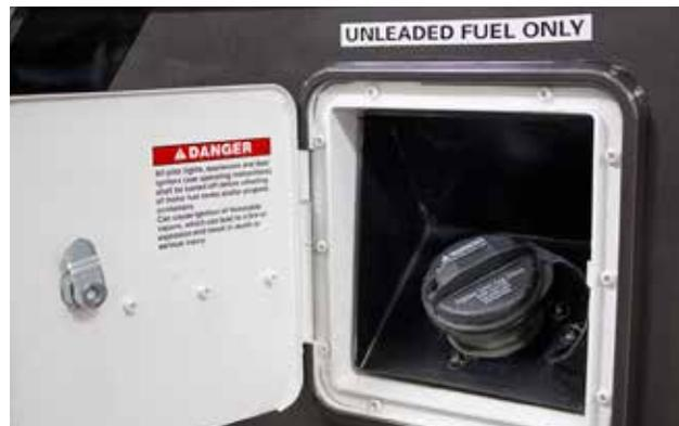
Fuel Tank Inlet for Fuel Transfer System
