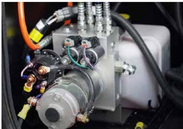
located near the entrance door or Monitor Panel on Class C motorhomes. The hydraulic pump is located in an outside service bay or rearward, between the chassis rails. The leveling system has been calibrated by the manufacturer and can be operated in Automatic or Manual Mode.
