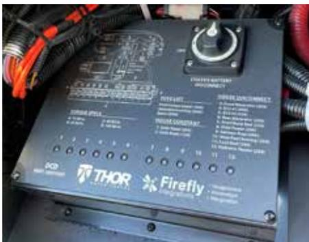
Master battery switch located on 12-volt circuit breaker panel.
