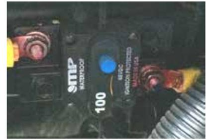
Typical Inverter Circuit Breaker located in the battery compartment.
