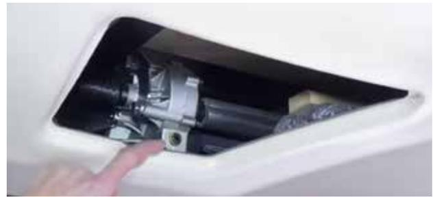
Figure 2. Motor Drive Socket.
