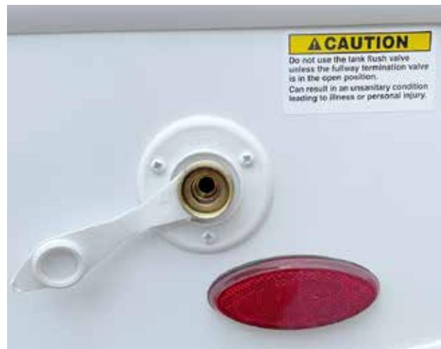
Typical black tank flush port located on the left side of the motorhome.
