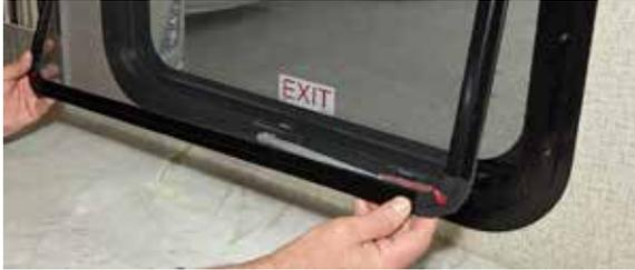
2. Push the red handle towards the window frame and lift it to release from the latch. Egress window latches vary in style, but all will be clearly marked with an 'Exit' label and be red in color.
