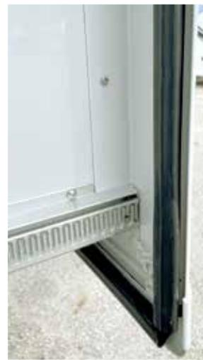
Keep slideout gear tracks and seals clean for proper maintenance and trouble-free operation
