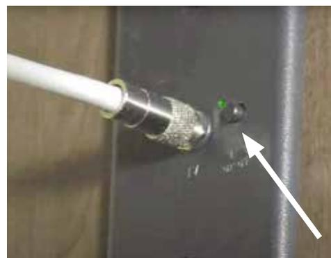
Antenna/Cable push-button selection switch with green LED
