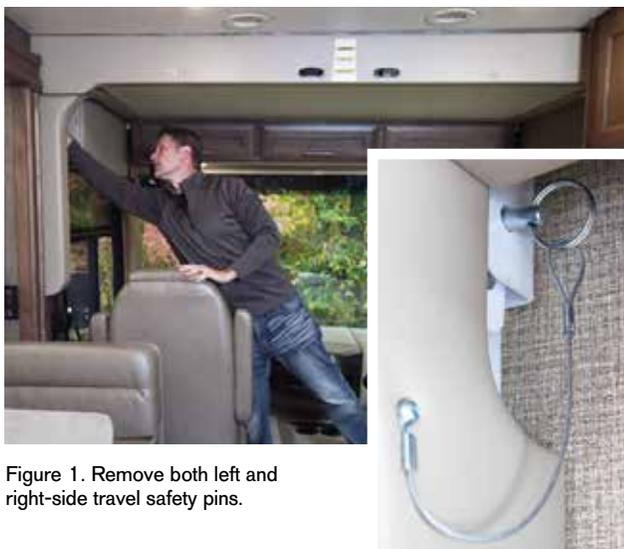
Figure 1. Remove both left and right-side travel safety pins.
