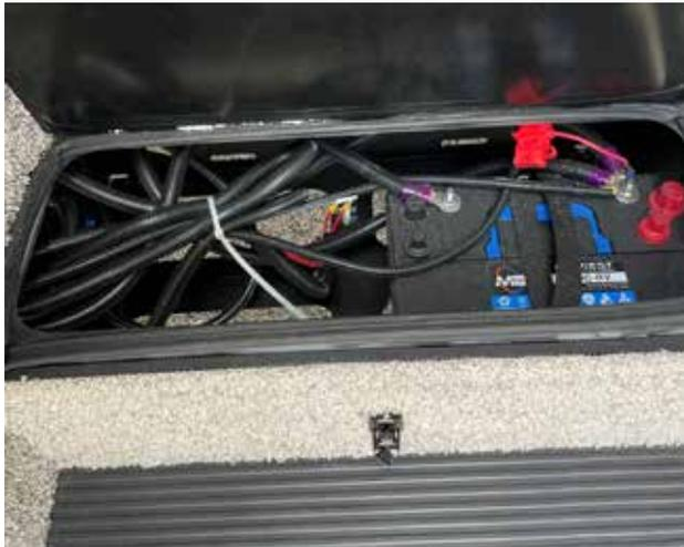
Typical Class C motorhome auxiliary battery location (under entrance step)
