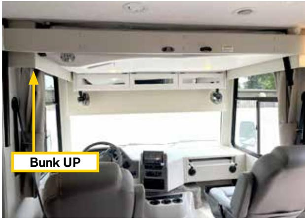
EuroLoft over-cab bunk in the up or stowed position (above). EuroLoft bunk in the lowered position (below).
