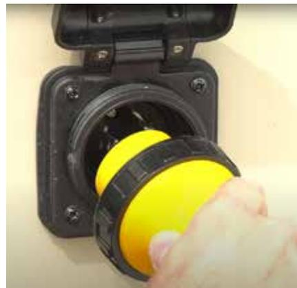
Attach the shore power cord to the motorhome by slipping the connector over the pins of the connection port. Give the connector a slight twist to the right, then spin-on the locking ring to secure the power cord to the motorhome.
