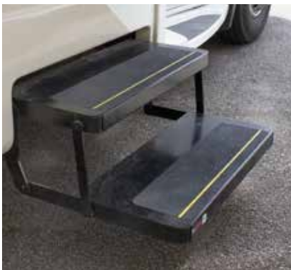
Typical powered entry steps.
