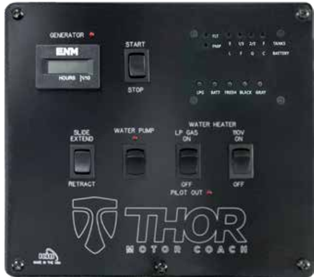
Typical Monitor Panel. Battery condition monitoring is usually located in the upper right corner.
