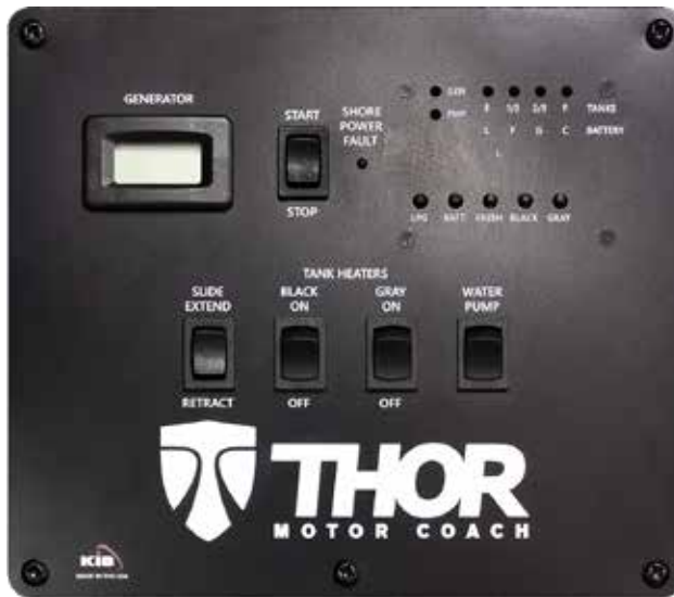
Typical Monitor Panel
