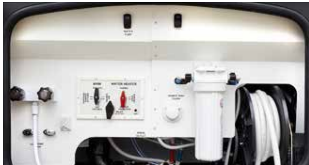
Water system panel for a Class A motorhome. Features vary by model and floor plan.
