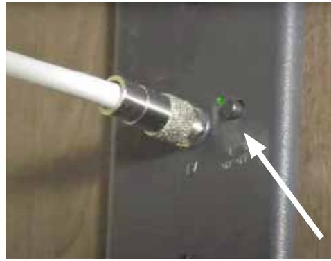
Antenna/Cable push-button selection switch with green LED
