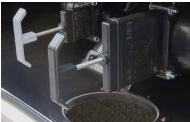
Typical termination valve configuration
