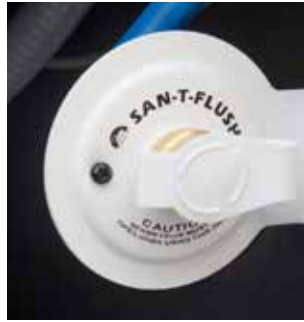
Typical black tank flush
