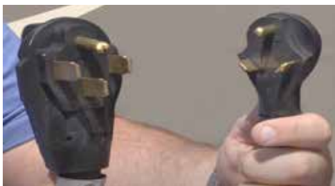
4-prong 50 amp shore power cord (left) and 3-prong 30 amp shore power cord (right)
