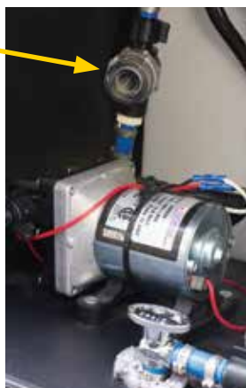
Water pump strainer
