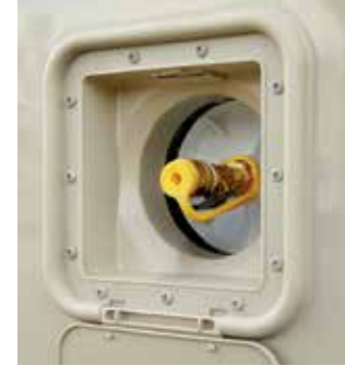
Typical external propane hook-up
