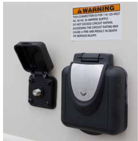
Typical park-supplied cable TV hook-up located on the driver's side of the motorhome. On some motorhome models, cable coax hookups are located on the freshwater panel or inside a left-side storage bay.
