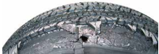
Tire pressure under and/or over inflation can cause severe tire failure
