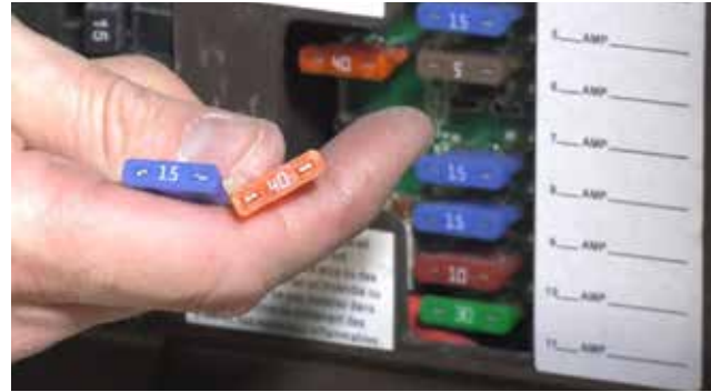
Automotive-type 12 volt fuses
