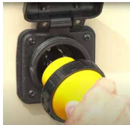
Typical shoreline power cord connection port
