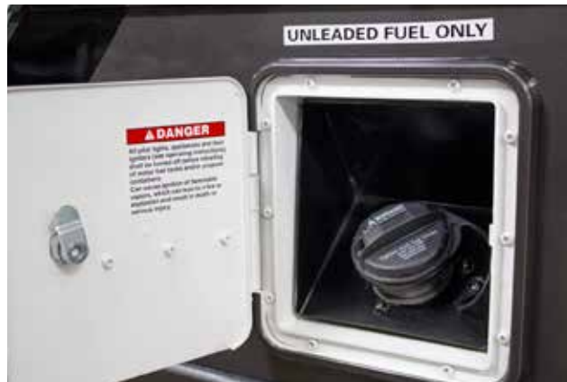
Fuel Tank Inlet for Fuel Transfer System
