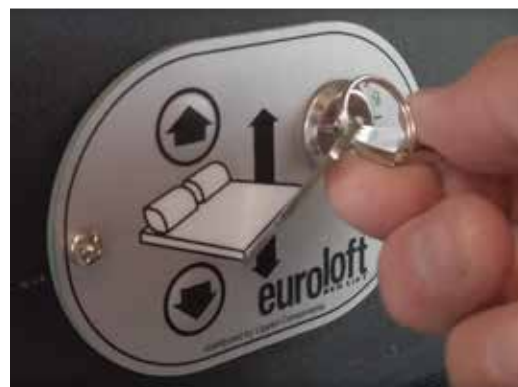
Typical Bed-lift switch panel. Styles may vary.
