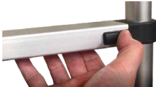
To Unlock: slide tabs towards the center of the rung. When a 'click' is heard, tab will lock OPEN, allowing section to collapse.
