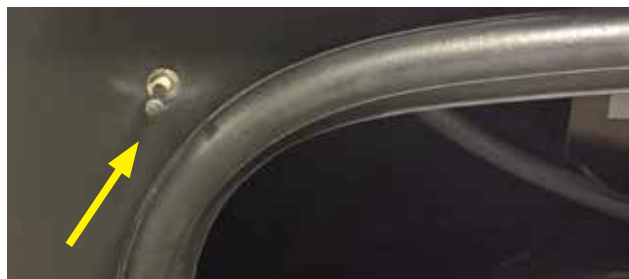
Fuel Pump Safety Lock-out Switch
