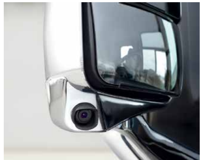
Mirrors are a vital component of safe motorhome operation. Convex mirror and side-view camera illustrated below.
