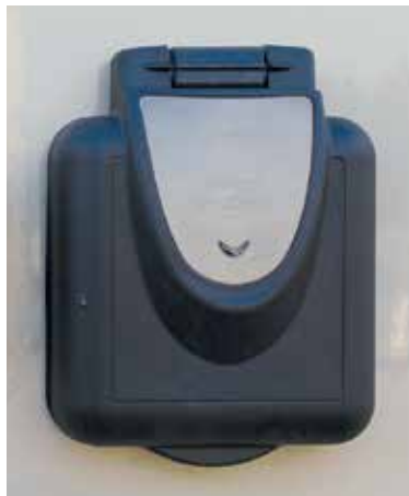
Typical shoreline power cord connection port
