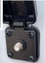
Typical park-supplied cable TV hook-up is usually located on the driver's side of the motorhome.
