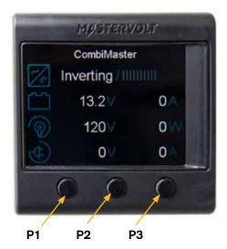
Mastervolt SmartRemote Inverter Monitor and Remote Controller
