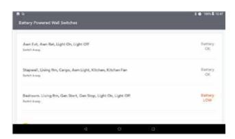
Battery powered wall switches settings. LOW indicates that the battery in the wall switch needs replacing.
