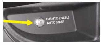
Auto-Start Control Button, located left of the steering wheel (RAM)
