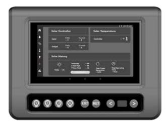
Illustration of BMPro touchscreen panel showing remote solar charging screen. Through the touchscreen panel, solar charging and battery charge condition can be monitored. Solar controller set-up is accessed through the Settings Menu.
