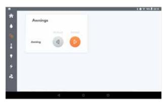
As a safety precaution, the RVMaster App will disable all motor control if the vehicle's ignition is ON. This safety feature prevents any accidental operation of the motors while you are driving the vehicle.
