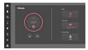
Set the desired air conditioned temperature from the Climate Menu on the Multiplex Touchscreen Controller.
