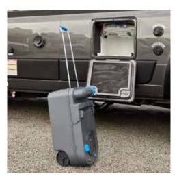
NOTE: Some Class B motorhomes have a bathroom with a cartridge toilet located at the rear of the vehicle. Access to the toilet cartridge is through the rear door.
