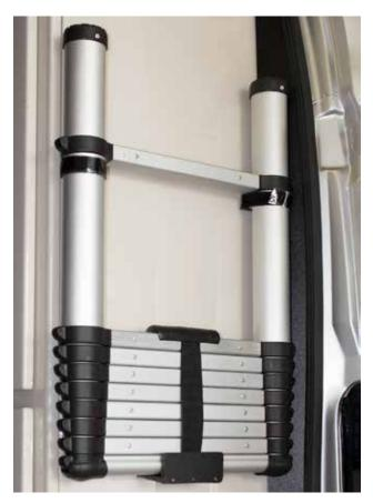
Collapsible ladder stowed behind rear door. The magnetic ladder bracket is stowed on the inside of the left-side rear door.
