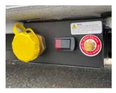
The main propane gas valve installed on this vehicle is controlled by an electrical solenoid. The actuation switch for the gas valve is located on the propane access panel, positioned along the lower left side of the vehicle. This panel also contains the propane tank fill port and a propane tank bleeder valve.
