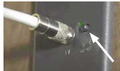
Antenna/Cable push-button selection switch with green LED
