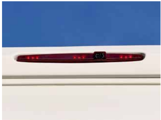
Typical rear vision camera located along the top rear edge of the motorhome.
