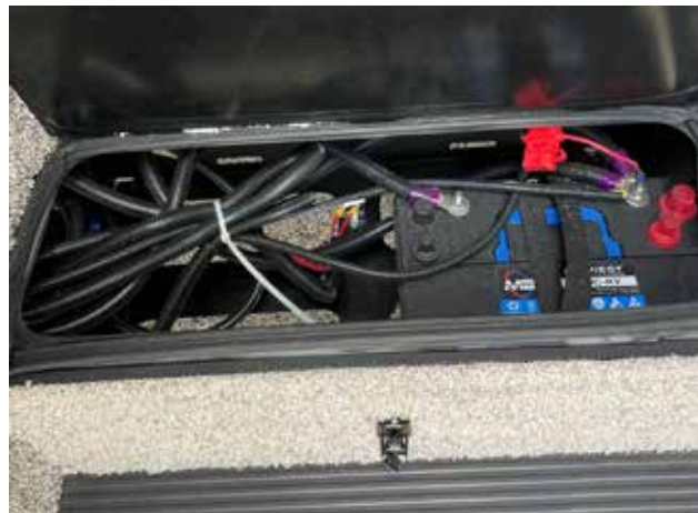
Typical Class C motorhome auxiliary battery location (under entrance step)
