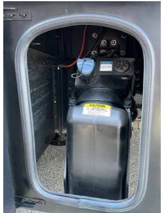
Typical DEF tank.
