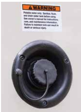
Typical freshwater gravity fill. Some fill caps may be located behind a lockable access panel.
