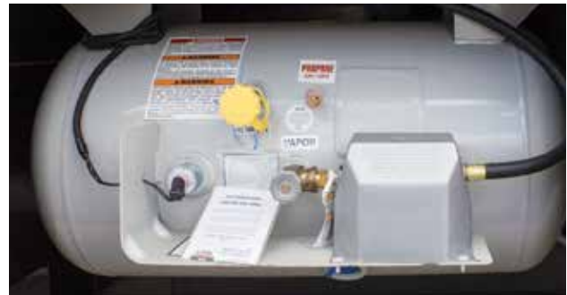
Typical permanently-installed RV propane tank with regulator
