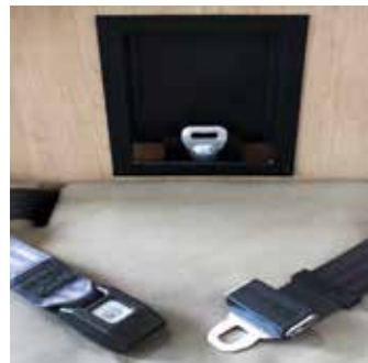
Child Safety Seat Anchor and lap belts. Strictly follow the installation directions of the child safety seat manufacturer when securing any child safety device to the motorhome.
