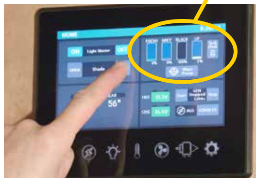
Multiplex touchscreen illustrating the tank monitoring display.
