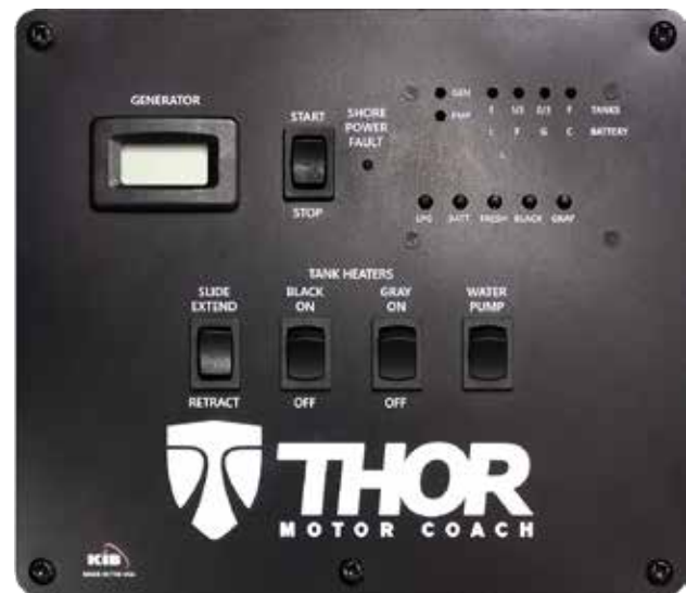
Typical Monitor Panel for non-multiplex electrical systems.
