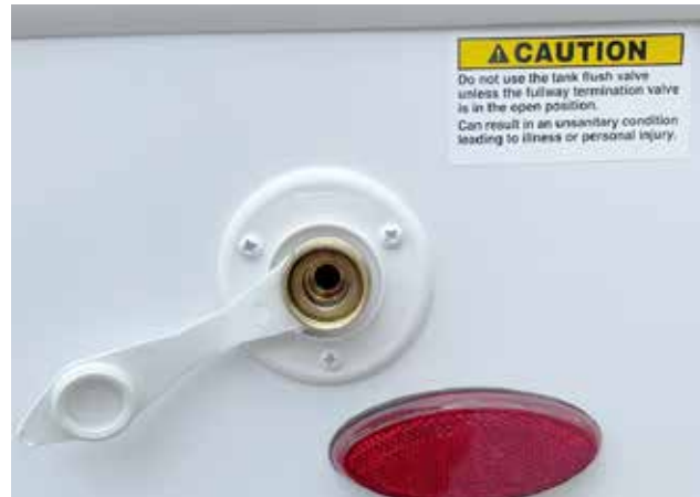
Typical black tank flush port located on the left side of the motorhome.
