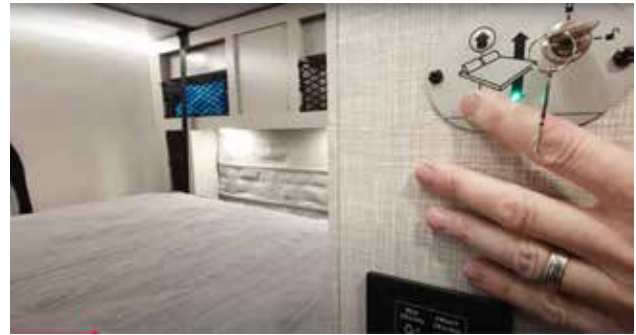
Figure 1: Lower bed by pressing DOWN arrow on the control panel.
