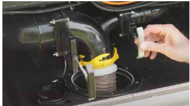
Closing the termination valves; close the gray valve first, then black valve.
