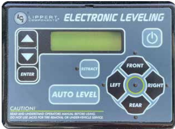
Typical Leveling Control Panel (above), which may contain an LCD read-out. Although differing in style, all LCI Leveling System Panels operate very similarly to one another. Hydraulic pump assembly (below).
