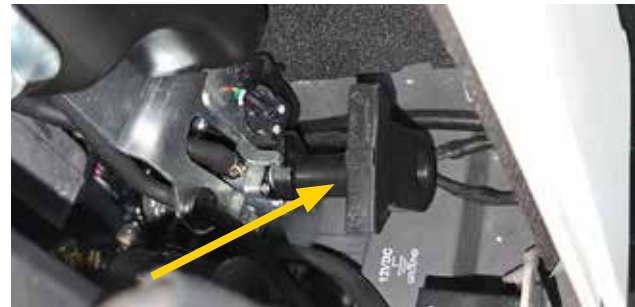
Fuel selection valve. Rotate for gasoline or propane operating fuel.
