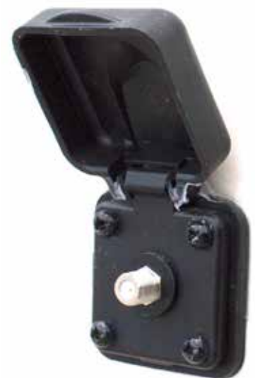
Typical park-supplied cable TV hook-up located on the driver's side of the motorhome. On some motorhome models, cable coax hookups are located on the freshwater panel or inside a left-side storage bay.
