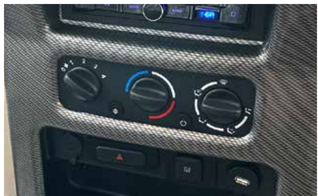
Typical Class A heating and air-conditioning dash controls
