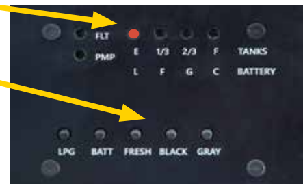
Monitor panel LED tank level display.
