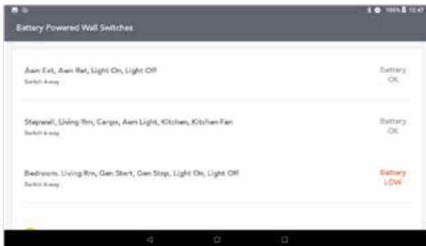
Battery powered wall switches settings. LOW indicates that the battery in the wall switch needs replacing.
