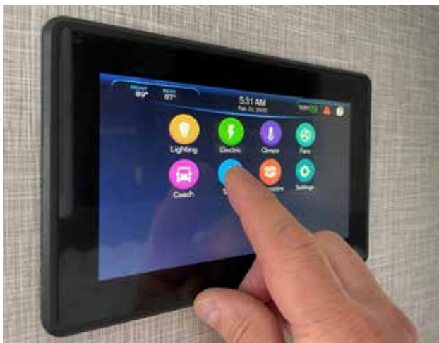
Typical multiplex main control panel. Features vary depending upon model and floor plan.
