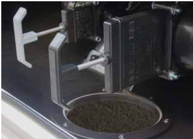
Typical termination valve configuration
