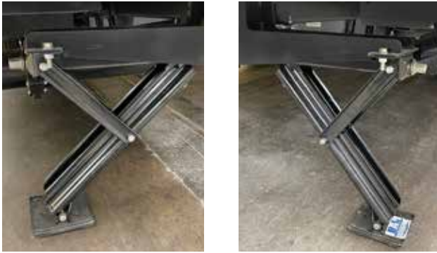
Typical left and right-side electric stabilizer jacks. For most systems, the left and right-side jacks operate independently.
