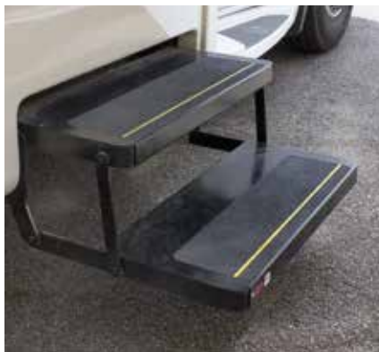
Typical powered entry steps. Depending upon motorhome model, steps may have one or more treads.
