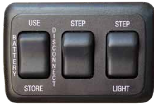
Typical powered entry step switch (center). Configuration may vary, however, all will be located near the entry door of the motorhome.
