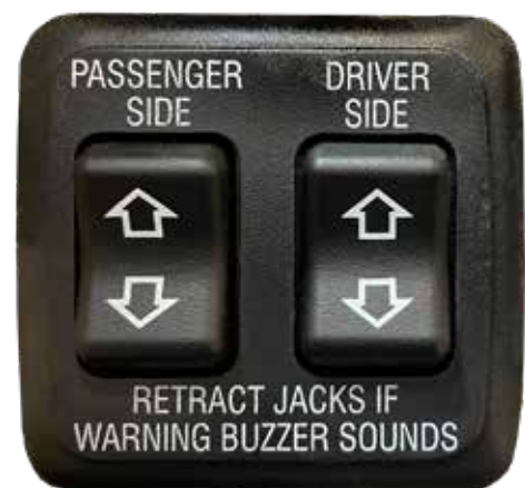
Typical Electric Stabilizer Switch Panel. The panel installed in your motorhome may differ from this illustration.
