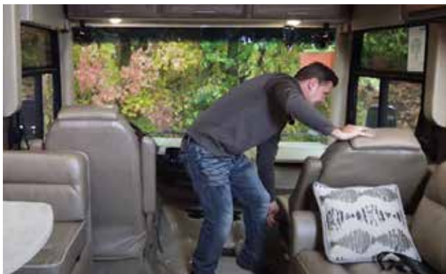
Figure 2. Recline both front seat backs before lowering the powered over-cab bunk.
