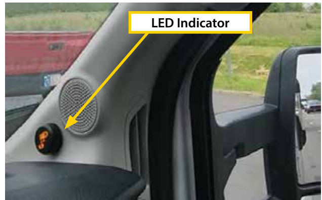
Blind Spot LED Indicator mounted on vehicle's left and right side 'A' pillars.
