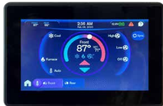
Typical multiplex control panels depicting climate control display
