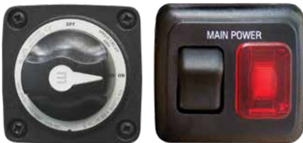
Typical master battery disconnect switches; rotary and rocker-type. Rocker-type switches control a relay, which in-turn, turns on and off power from the auxiliary battery(ies).
