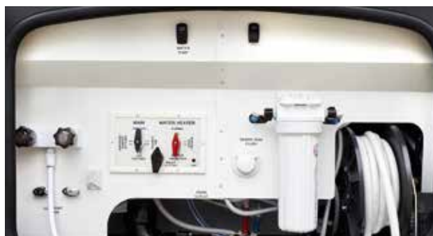
Water system panel for a Class A motorhome.
