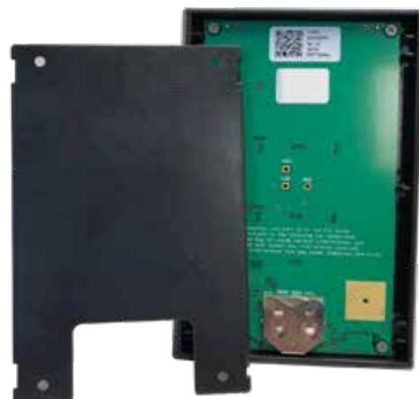
NOTE: To access the battery, pry the switch from the wall mounting cradle to expose the battery compartment on the rear of the switch and replace the #2032 coin-cell battery.
