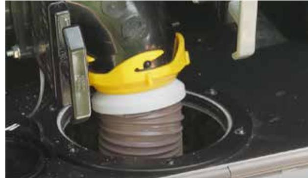
Sewer hose connected to the motorhome's wastewater outlet.
