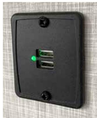
**NOTE:** Charging ports are generally powered by the motorhome's 12-volt DC system. The Main Battery Switch must be ON to activate USB Charging Ports.
