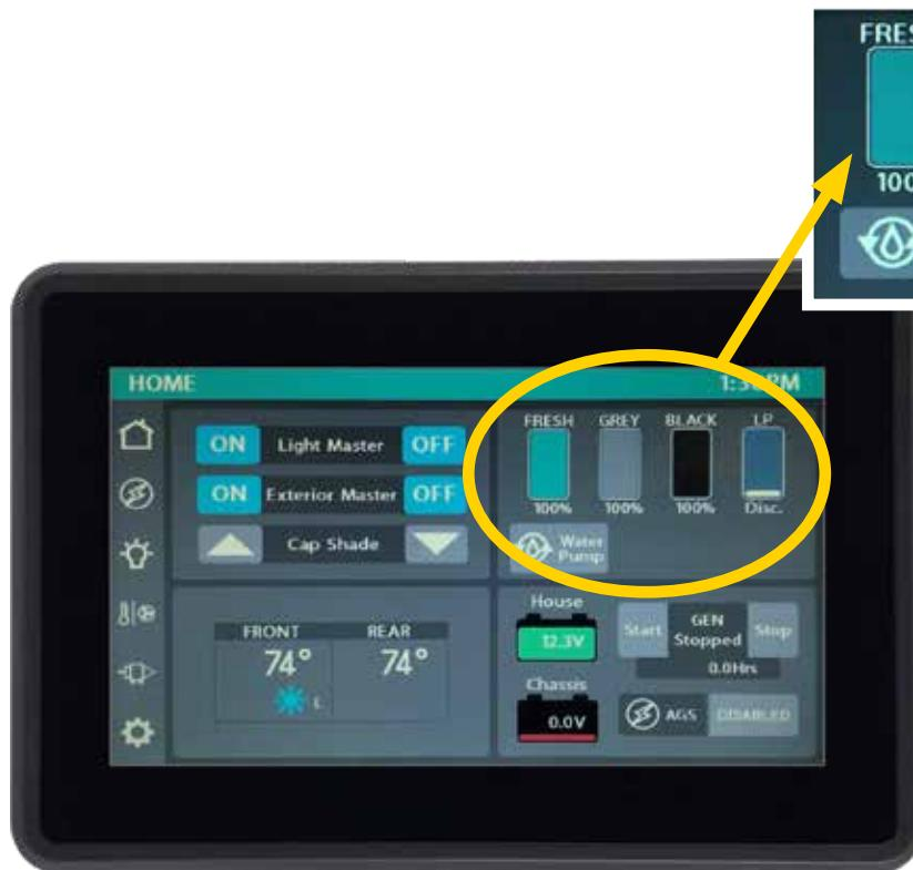
Multiplex touchscreen illustrating the tank monitoring display.
