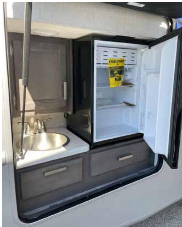
Examples of optional exterior kitchens. Depending on floor plan options, exterior kitchens may include: cabinet storage, refrigerator, sink with hot and cold running water (see above), pull-out gas griddle, water sprayer with hot and cold water (see below).
