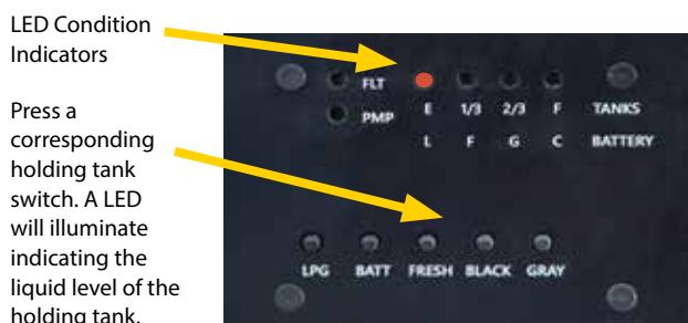
Monitor panel LED tank level display.
