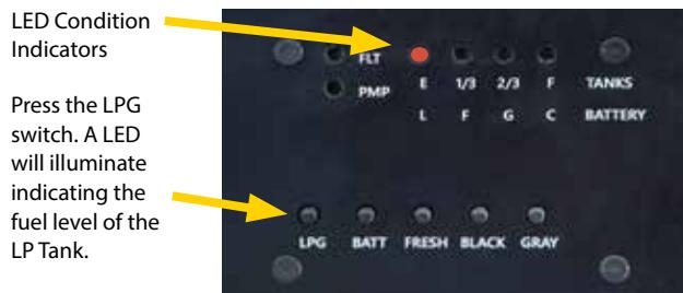
Monitor panel LED tank level display.
