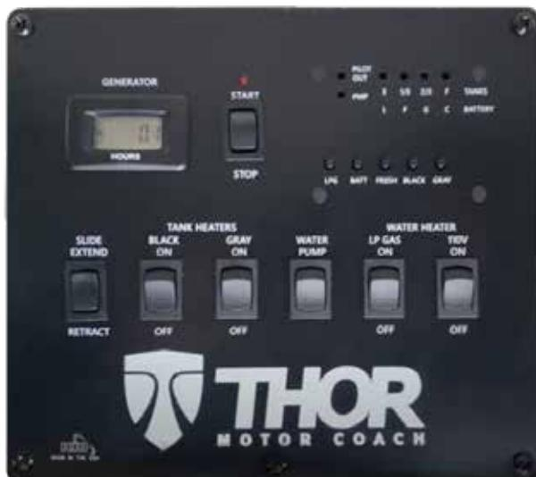
The slideout control switch supplied on your motorhome may be located on the main system panel (illustrated above) or found on the Slides/Awnings menu screen of a multiplex touchscreen panel (below). Some floor plans will have slideout extend and retract control switches mounted on a wall near the slideout.
