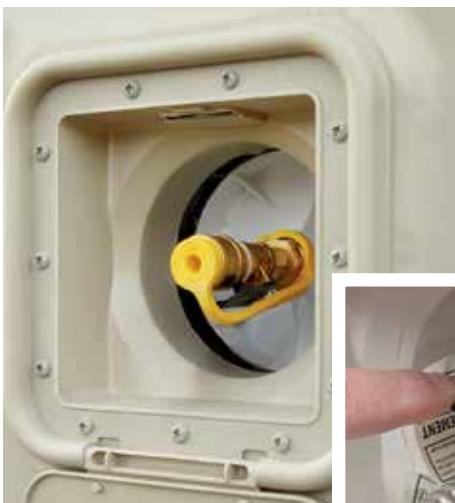
(Above) Typical external propane hook-up port. (Right) manual shut-off valve.
