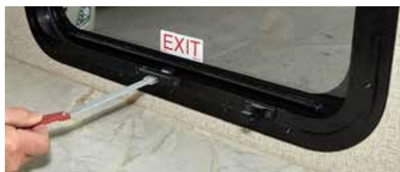
4. Push the handle, which opens the window. If the window pane is stuck, pushing on the window pane's frame may be necessary in order to free it from the window seal. Continue to push the handle until it is completely clear of the slot in the window frame.
