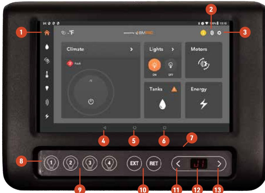
**NOTE:** Lighting and motor control switches (#9 and 10) can be operated immediately after the Touchscreen Panel is powered. It is not necessary to wait for the Master App to launch (boot-up).
