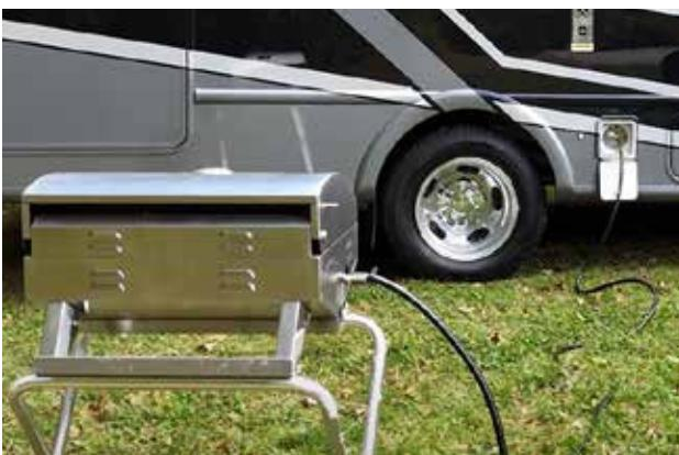
Although designed for a wide variety of outdoor LP uses, the External LP Hook-up port provides a particularly convenient LP connection source for a propane griddle.
