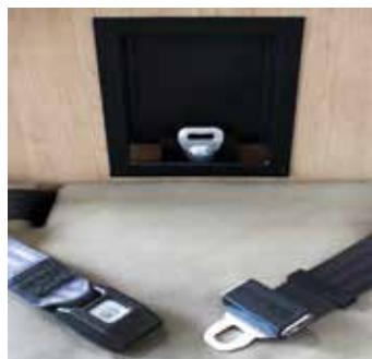
Child Safety Seat Anchor and lap belts. Strictly follow the installation directions of the child safety seat manufacturer when securing any child safety device to the motorhome.
