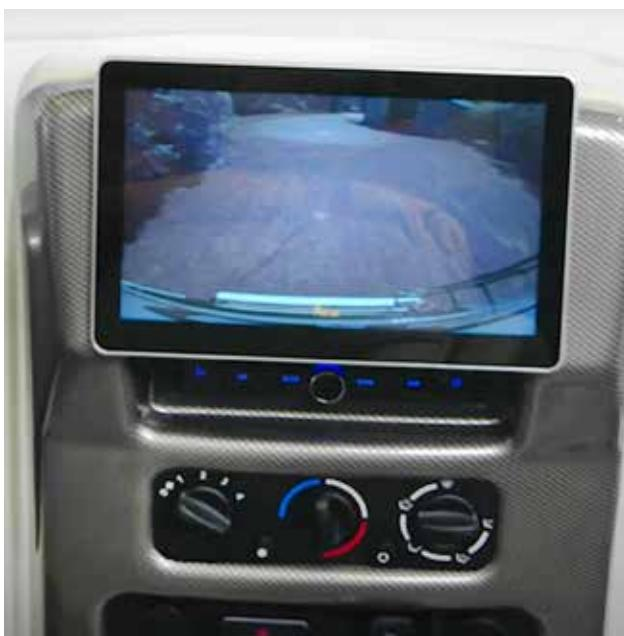
Typical dash radio with camera monitor
