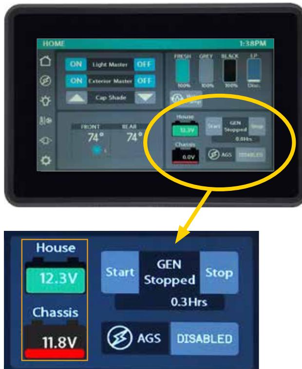
Typical multiplex main control panel. Basic electrical system monitoring is usually located on the main menu (Home) screen.
