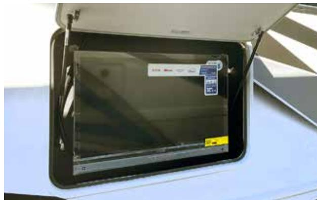
Most TMC Class A motorhomes and select Class C motorhomes are equipped with a camp-side external TV.
