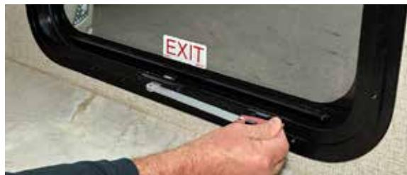
3. Rotate the handle until it is perpendicular to the window frame.
