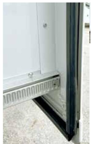
Keep slideout gear tracks and seals clean for proper maintenance and trouble-free operation
