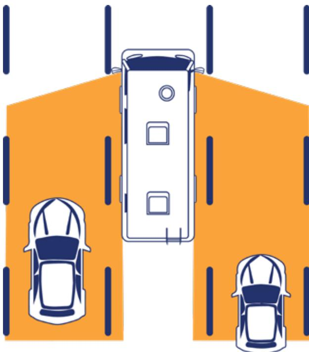
The Blind Spot Detection System is programmed to detect Department of Transportation (DOT) approved motor vehicles: motorcycles, cars, and trucks. It will not detect pedestrians, bicycles, and animals.
