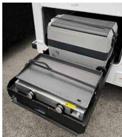
Mounted on a convenient pull-out tray (along with the gas griddle), the 40 quart, 12 volt cooler/freezer contains two temperature controlled cooling zones and storage baskets. The zone divider can be removed, creating a large, single cooling or freezing area.
