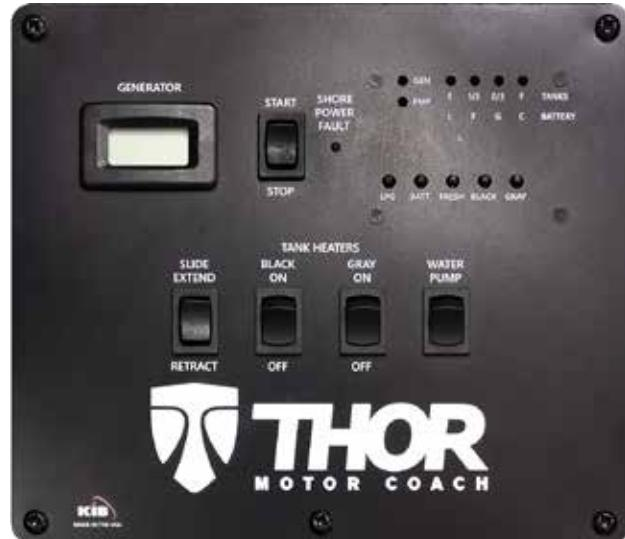
Typical Monitor Panel for non-multiplex electrical systems.
