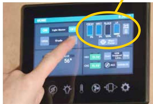
Multiplex touchscreen illustrating the tank monitoring display..
