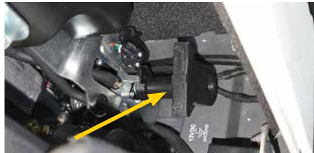
Fuel selection valve. Rotate for gasoline or propane operating fuel.
