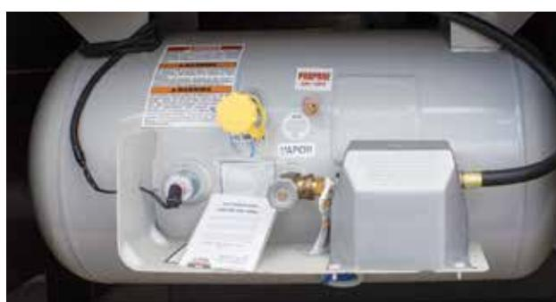
Typical permanently-installed RV propane tank with regulator
