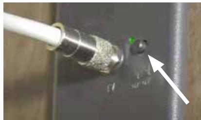
Antenna/Cable push-button selection switch with green LED
