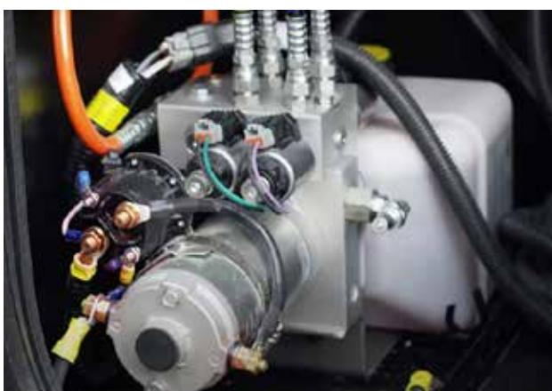
The Control Panel is conveniently located near the driver's seat in Class A motorhomes. This control panel is often located near the entrance door or Monitor Panel on Class C motorhomes. The hydraulic pump is located in an outside service bay or rearward, between the chassis rails. The leveling system has been calibrated by the manufacturer and can be operated in Automatic or Manual Mode.
