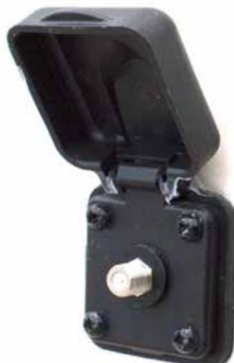
Typical park-supplied cable TV hook-up located on the driver's side of the motorhome. On some motorhome models, cable coax hookups are located on the freshwater panel or inside a left-side storage bay.
