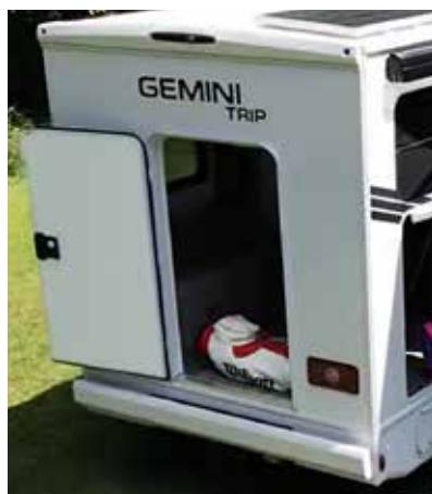
Typical rear cargo door. For this particular floor plan, the photo illustrates rear bed in a stowed (up) position.
