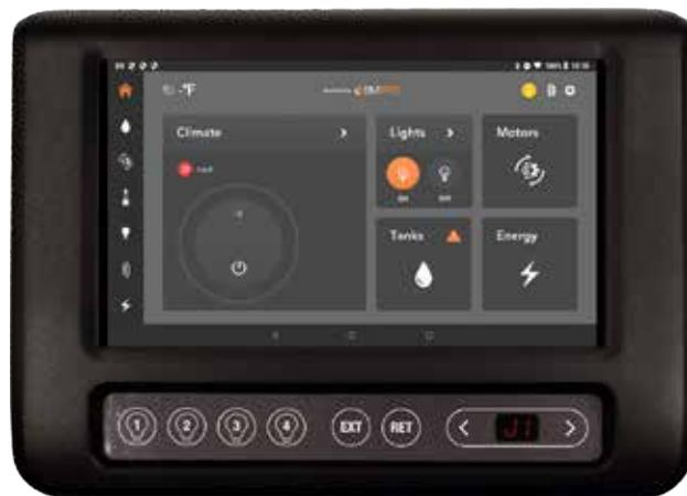
A sidebar located along the left edge of the touchscreen, provides easy navigation to all the main screens of the RVMaster App.
