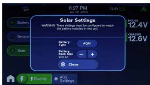
Figure 4: Solar settings screen.
