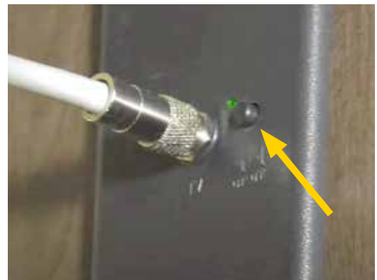
Antenna/Cable push-button selection switch with green LED.
