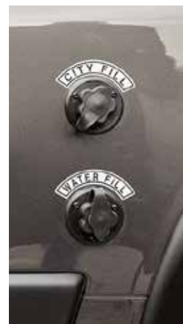
City water connection. The water ports on Class B motorhomes vary in type and location due to floor plans and available features.
