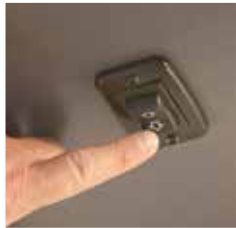
Motorized bench seat and actuation switch. For some models the rear bench seat is manually operated only.
