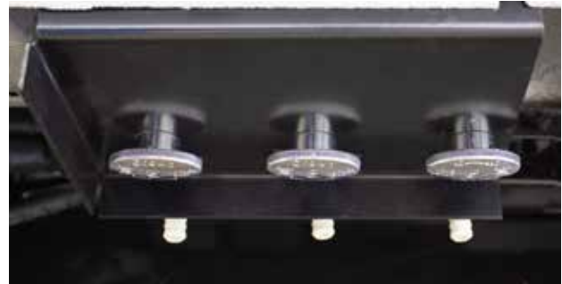
Low point drain valves are typically located underneath the left-side rocker panel
