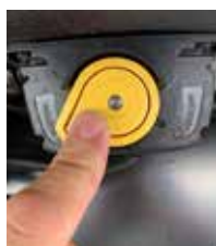
Safety Relay rotated to the ON position. Depress the center to engage the safety relay
