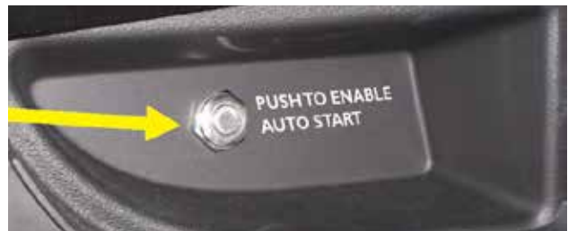
Auto-Start Control Button, located left of the steering wheel. Press this button to enter AES system monitoring mode.
