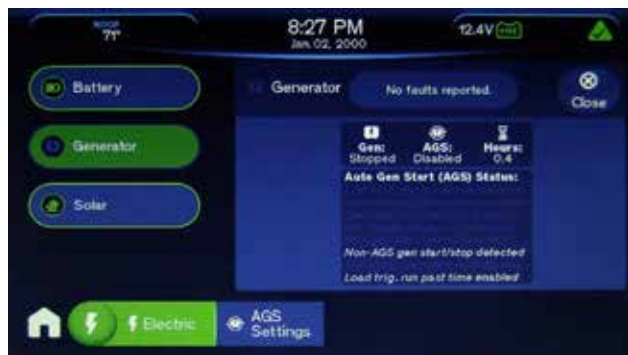
Figure 2: Generator Status Screen.
