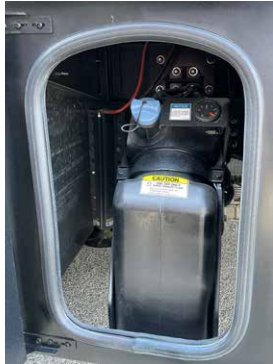
Typical DEF tank.
