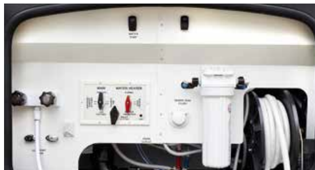
Water system panel for a Class A motorhome. Features vary by model and floor plan.
