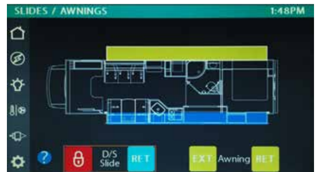
The slideout control switch supplied on your motorhome may be located on the main system panel (illustrated above) or found on the Slides/Awning menu screen of a multiplex touchscreen panel (below).
