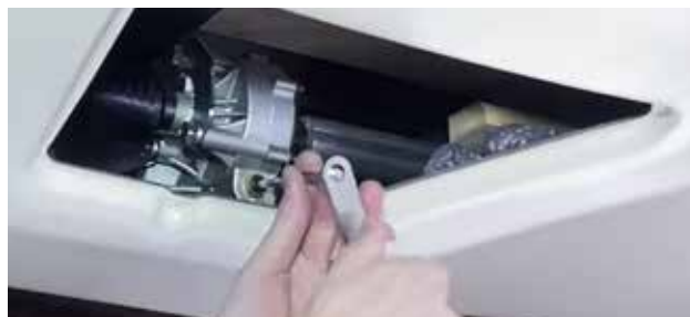
Figure 3. Insert Crank. Turn clockwise to raise, counter-clockwise to lower the bed.
