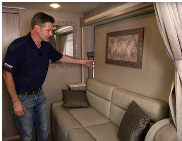
Powered Murphy Bed; stowed (above) and lowered position (below)
