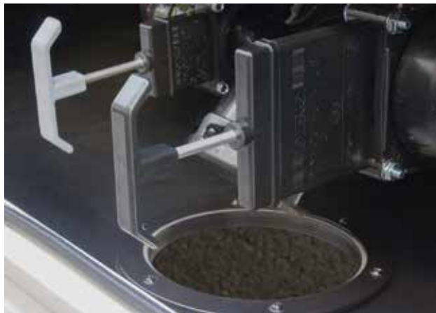
Typical termination valve configuration
