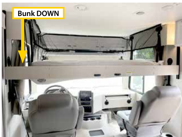
EuroLoft over-cab bunk in the up or stowed position (above). EuroLoft bunk in the lowered position (below).
