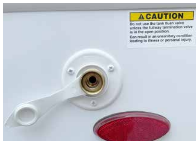
Typical black tank flush port located on the left side of the motorhome.
