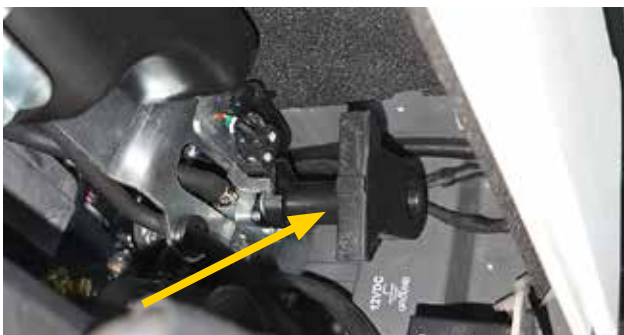
Fuel selection valve. Rotate for gasoline or propane operating fuel.
