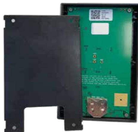
Typical multiplex wireless switch panel. Battery compartment access (below).
