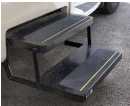
Typical powered entry steps. Depending upon motorhome model, steps may have one or more treads.
