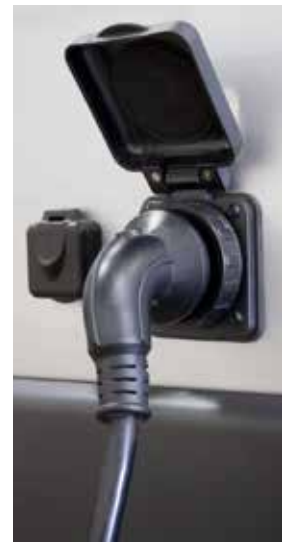
Typical shoreline power cord connection port
