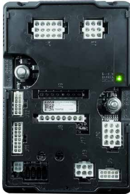
Firefly Integrations system control board
