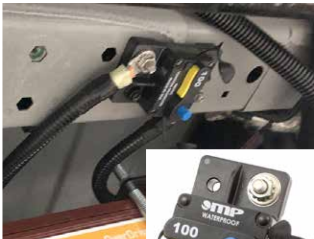
Typical 100 Amp Inverter Circuit Breaker located on a frame member underneath the vehicle, near the battery trays.
