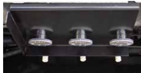
Low point drain valves are typically located underneath the left-side rocker panel
