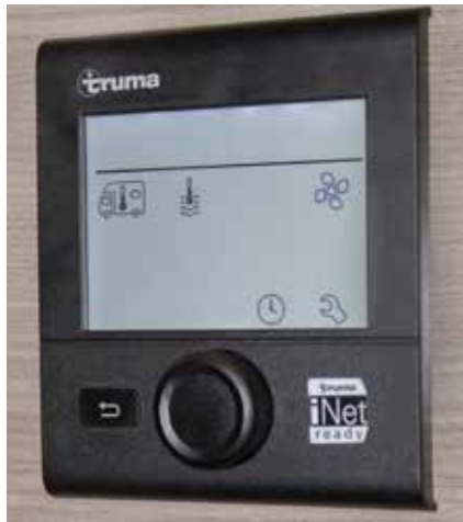
Combination Furnace/Water Heater wall- mounted controller
