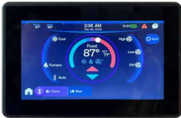
Set the desired air conditioned temperature from the Climate Menu on the Multiplex Touchscreen Controller.
