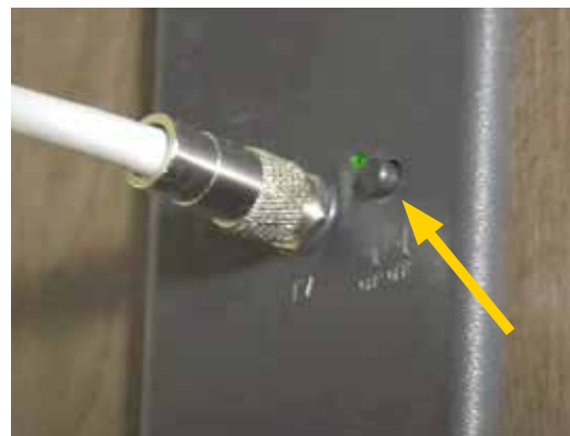
Antenna/Cable push-button selection switch with green LED
