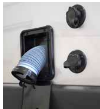
City water fill connection, along with a storage chamber for the sewer hose. This image for reference only. The water ports on Class B motorhomes vary in type and location due to floor plans and features.
