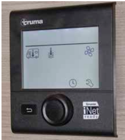
Combination Furnace/Water Heater wall- mounted controller
