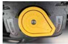
Safety Relay in the OFF position. 400 and 460 Ah systems have one safety relay, while 800 and 920 Ah systems have two safety relays, one for each battery pack.
