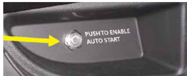
Auto-Start Control Button, located left of the steering wheel (RAM)
