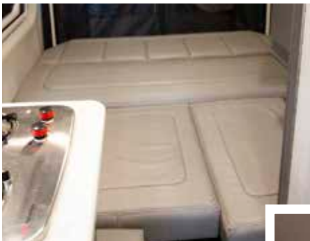
Motorized bench seat and actuation switch. For some models the rear bench seat is manually operated only.
