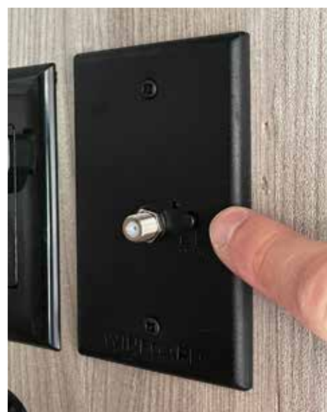
Antenna/Cable push-button selection switch with green LED
