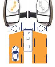
3. Vehicle in blind spot, turn signal is ON:
