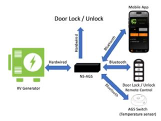
Class C AGS system diagram, including smartphone remote operation and wireless cab door locks.
