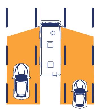
The Blind Spot Detection System is programmed to detect Department of Transportation (DOT) approved motor vehicles: motorcycles, cars, and trucks. It will not detect pedestrians, bicycles, and animals.
