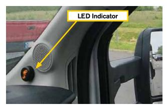
Blind Spot LED Indicator mounted on vehicle's left and right side 'A' pillars.
