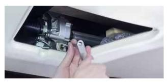
Figure 3. Insert Crank. Turn clockwise to raise, counter-clockwise to lower the bed.
