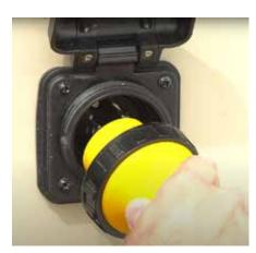
Attach the shore power cord to the motorhome by slipping the connector over the pins of the connection port. Give the connector a slight twist to the right, then spin-on the locking ring to secure the power cord to the motorhome. ELECTRICAL SYSTEM
