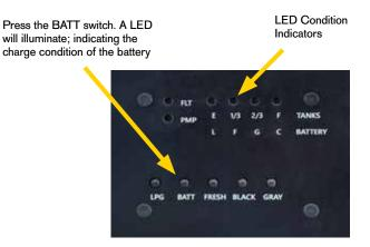
Battery Condition LEDs:
