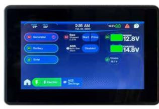
Typical multiplex main control panel. Electrical system monitoring is usually located on the main menu (Home) screen.
