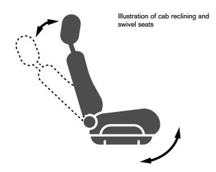
For comfort and convenience, your motorhome may be equipped with tilt and swivel seats in the cockpit area. These features are designed to only be used when the motorhome is parked. Before travel or moving the motorhome, ensure all front seat backs are returned to an up-right position, swiveled, and locked in their forward-facing position.
