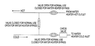
Water Heater Bypass Valve diagram
