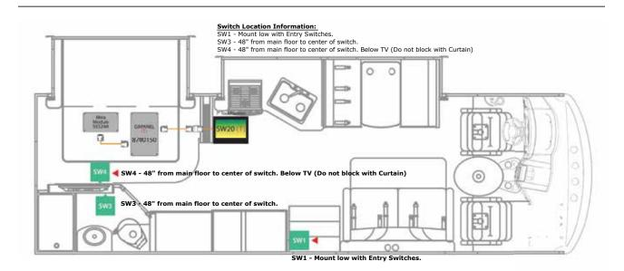
Wiring illustration (below) of a typical multiplex system; consisting of main touchscreen control panel, wireless room switches, and electrical power control panels and modules.
