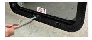
4. Push the handle, which opens the window. You may need to push on the window glass to free it from the window seal. Continue to push the handle until it is completely clear of the slot in the window frame.
