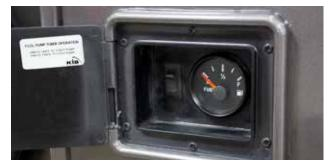
Fuel Pump Switch and Fuel Gauge for Fuel Transfer System
