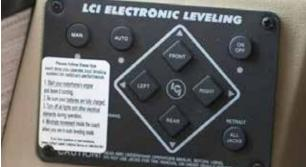
Typical Leveling Control Panels (above), which may contain an LCD read-out. Hydraulic pump assembly (below)
