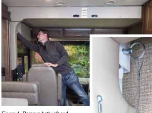
Figure 1. Remove both left and right-side travel safety pins.
