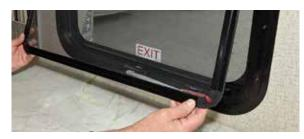
2. Push the red handle towards the window frame and lift it to release from the latch. Egress window latches vary in style, but all will be clearly marked with an 'Exit' label and be red in color.
