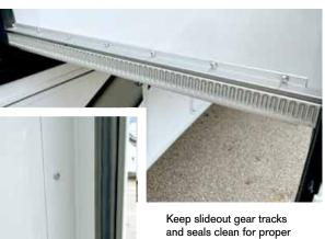
Keep slideout gear tracks and seals clean for proper maintenance and trouble-free operation
