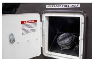
Fuel Tank Inlet for Fuel Transfer System
