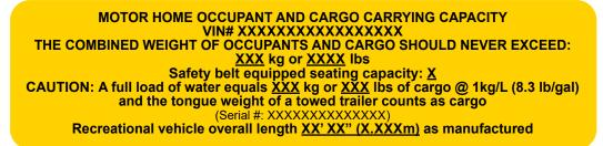
Typical Motorhome Occupant and Cargo Carrying Capacity Label
