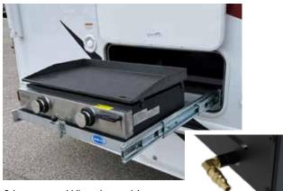
2-burner gas griddle and gas quickdisconnect coupler.
