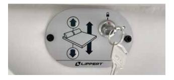
4. PRESS and HOLD the arrow-shaped DOWN Position switch. A green LED light on the control panel will turn ON in the direction of bed is moving. The bed will stop automatically when it reaches the pre-set stop position.
