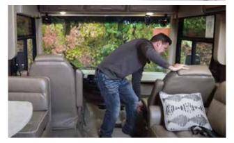
Figure 2. Recline both front seat backs before lowing the powered over-cab bunk.
