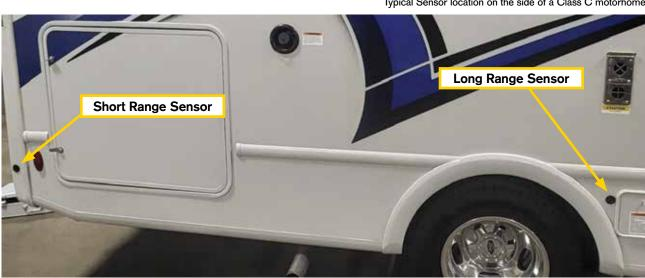
Typical Sensor location on the side of a Class C motorhome.
