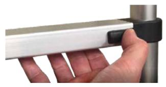
To Unlock: slide tabs towards the center of the rung. When a 'click' is heard, tab will lock OPEN, allowing section to collapse.
