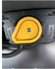
Safety Relay engaged, turning ON the battery pack
