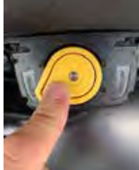
Safety Relay rotated to the ON position. Depress the center to engage the safety relay
